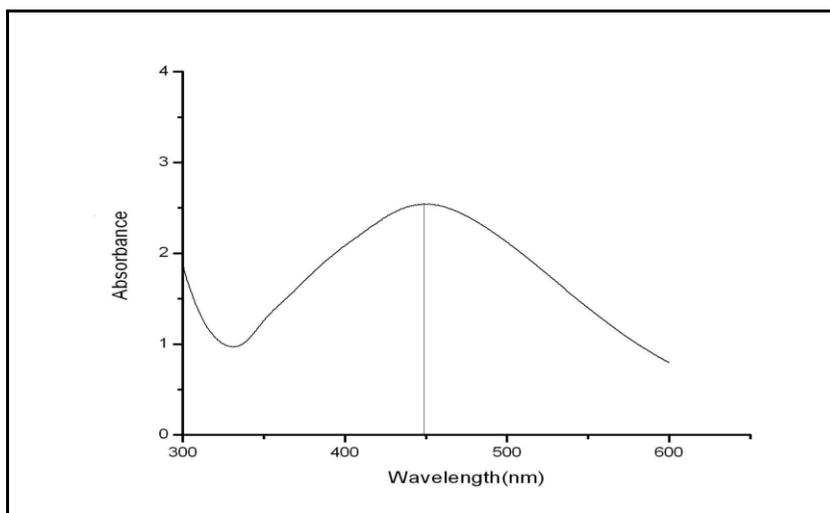
**Fig.1. UV-Vis absorption spectra of 'Green' Silver nanoparticles synthesized by addition of Grape fruit extract with 10mM silver nitrate aqueous solution.**
