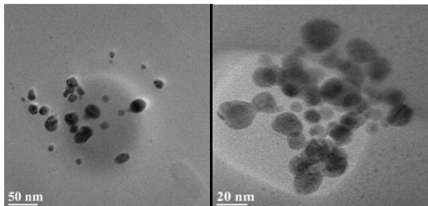
Fig.3.1. TEM images of silver nanoparticles synthesized by using Grape fruit extract
