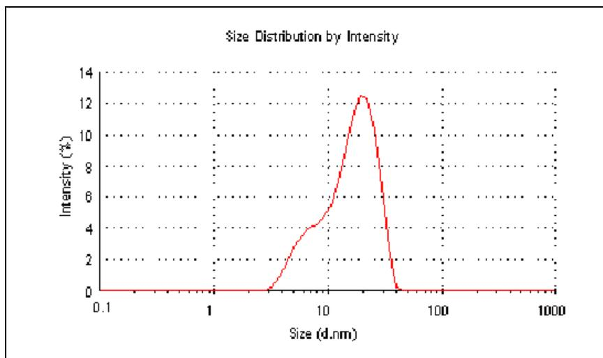
Fig.2. DLS showing mean average size of silver nanoparticles as 19 nm
