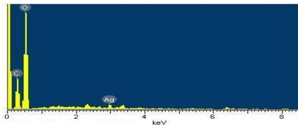
Figure.4. EDX curve with three dominant peaks for C, O and Ag respectively
